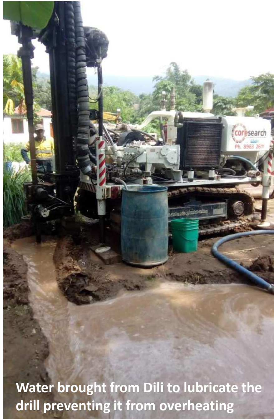
Using drill size 8-1/2" to hit bedrock
